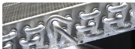
Aluminum tube and tube sheet after 500 hour salt spray.
