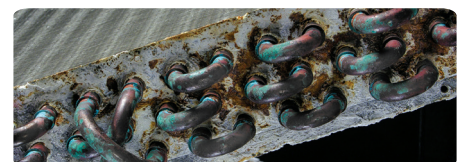
Copper tube and galvanized tube sheet after 500 hour salt spray.
